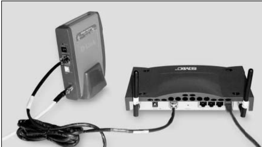
(Left: Cable Modem Right: Wireless router with LAN Ports- Ethernet Cables)
